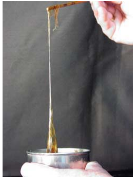
Fig. 12 Burnt plate oil--Linseed oil that has been heated to ignition (400°C.) and has become thick and viscous.
