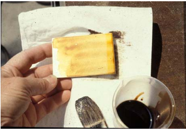
Fig. 3 Application of a coating of bitumen (pine tar pitch) on a polished bronze 85:5:5:5 plate.
